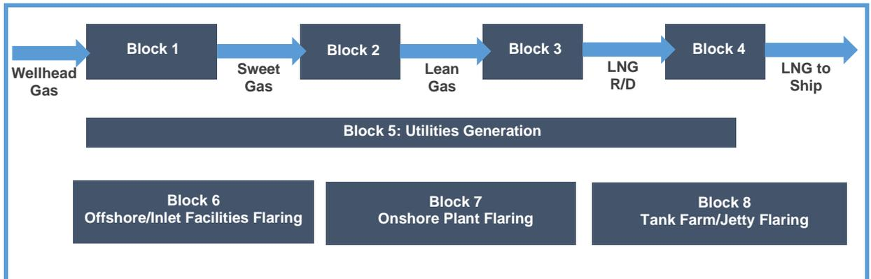
Figure 10.2. Example process block breakdown for an LNG plant
